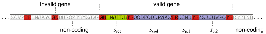
Fig. 2. In order to encode a gene parameter p , genes must have two additional sequences s_{p,1} and s_{p,2} . Thus, a valid gene with one gene parameter has four sequences separated by tokens ‘TE’. The token ‘GN’ to the left of the valid gene is not followed by the necessary four tokens ‘TE’, thus it is not coding.
